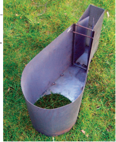
Photo 2. Metal box trap with a removable resting chamber for the fry.
