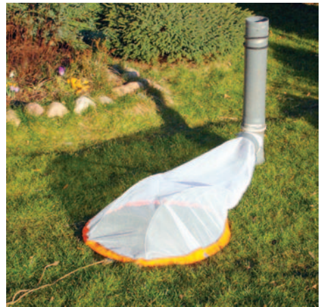
Photo 1. Medium cap trap with a vertical tube (metal hoop circumference – 75 cm).
